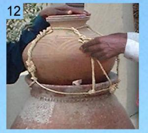
Using the nail make one hole by hand in the bottom of the mutka to one side.
