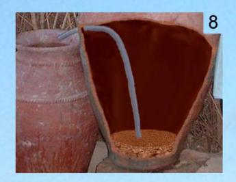
Put in sand, sieved through the middle size mesh and washed, to this level.
